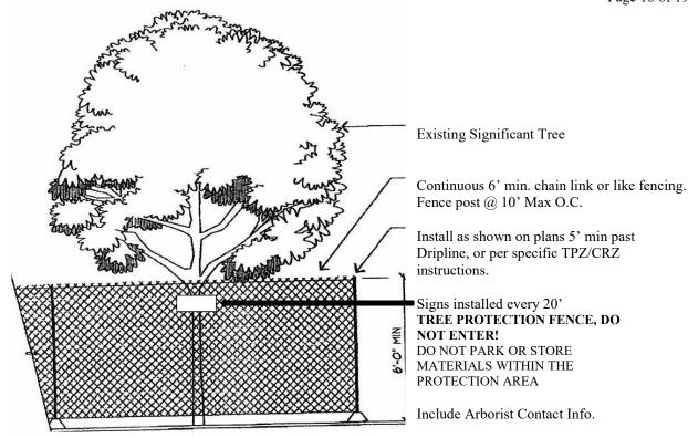
Six-foot high temporary chain link (or like material) fencing shall be installed as shown on plans. Fencing shall be installed prior to construction activity and remain in place until construction is completed. Fencing panels are recommended. Fencing shall completely encircle the tree(s). Install fence posts using pier blocks. Avoid driving posts or stakes into major roots.
